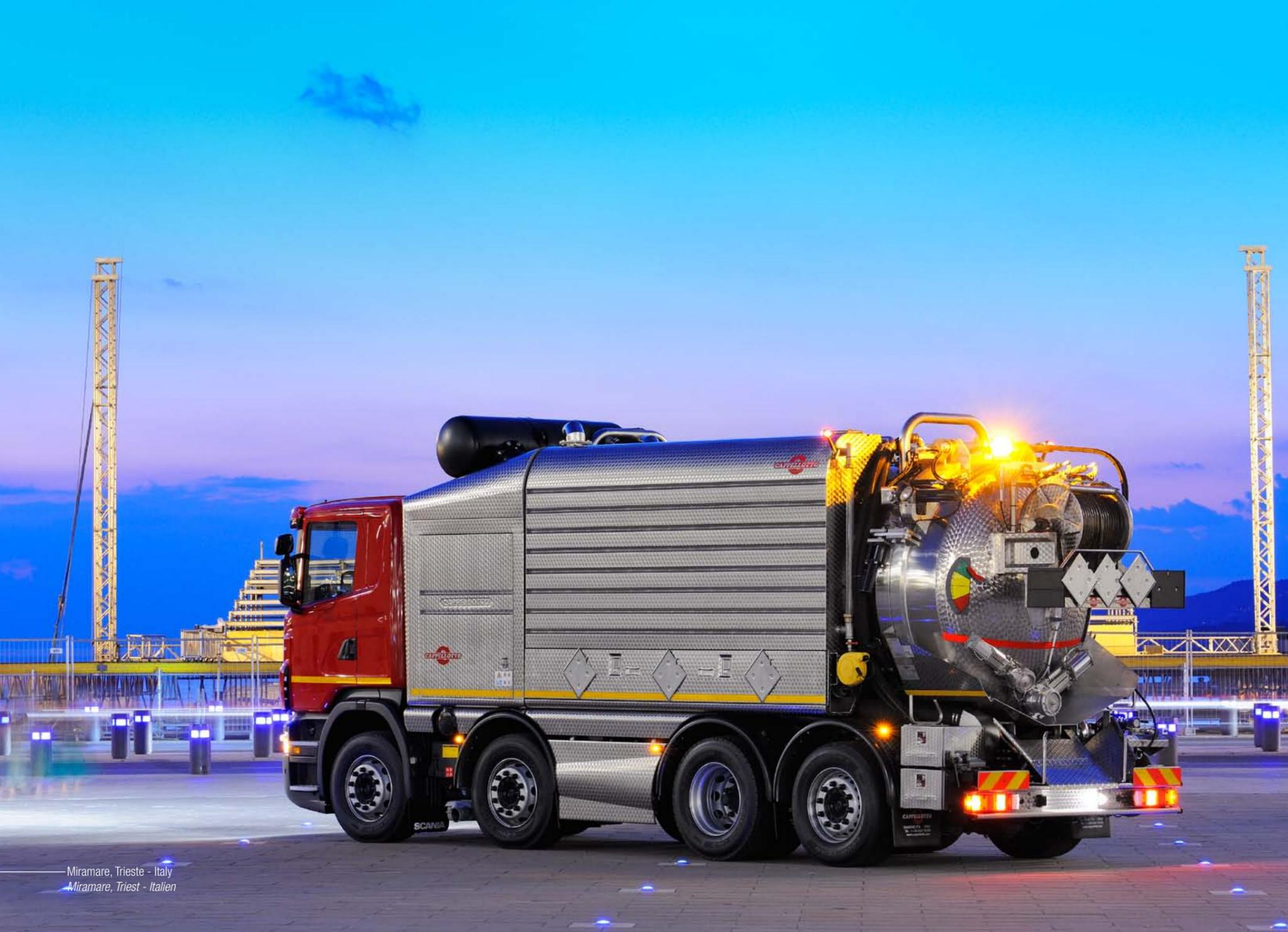
Connection profiles custom-made for better aerodynamics, less dirt build-up and easier access to the controls.
